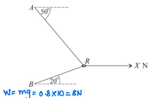
A light inextensible string has its ends attached to two fixed points  $A$  and  $B$ , with  $A$  vertically above  $B$ . A smooth ring  $R$ , of mass  $0.8\text{ kg}$ , is threaded on the string and is pulled by a horizontal force of magnitude  $X$  newtons. The sections  $AR$  and  $BR$  of the string make angles of  $50^\circ$  and  $20^\circ$  respectively with the horizontal, as shown in the diagram. The ring rests in equilibrium with the string taut. Find
