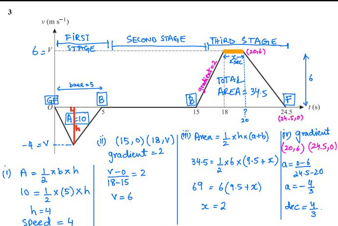
The diagram shows the velocity-time graph for a lift moving between floors in a building. The graph consists of straight line segments. In the first stage the lift travels downwards from the ground floor for 5 s, coming to rest at the basement after travelling 10 m. (area = 10)
